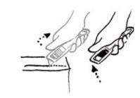
SECUNORM: high degree of safety thanks to the automatic blade retraction As with the fully automatic blade withdrawal, only you need to release the slider or lever during cutting.
